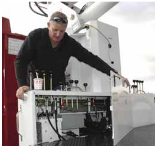
A panel is easy to open to access the controls for repairs on the Elliott 1560F.
