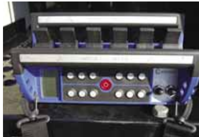
National’s NBT14 features radio-remote controls as standard.
