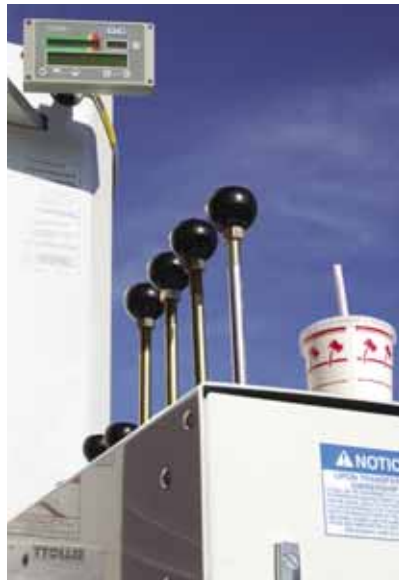
Elliott turns to single-axis controllers for reliability. At the operator station is a cup holder and the optional Greer LMI display.
