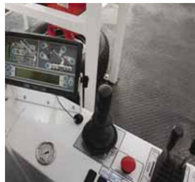
Altec uses pilot-operated joysticks and offers its LMAP rated capacity limiter with area protection as standard.
