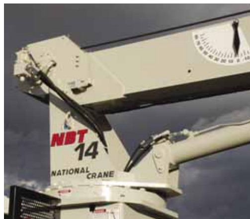
The NBT14's compact boom butt reduces tailswing.
