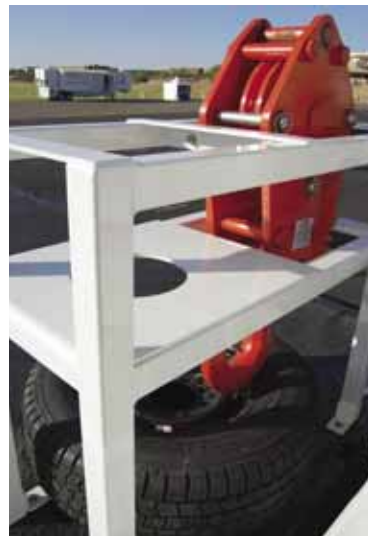
Integral storage systems for the block and outrigger pads are included on the Altec AC18-70B.
